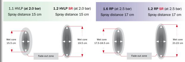
Standard nozzles with wet, compact core. SR nozzles with wide-streched core.
